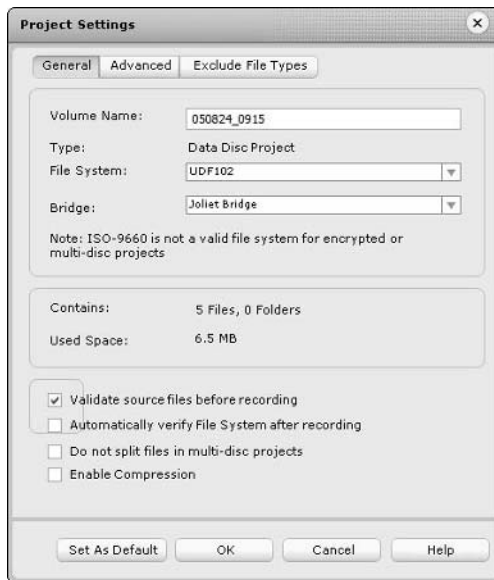
Figure 3-10: Review and change the settings for your new Data Disc project in the Project Settings dialog box.
